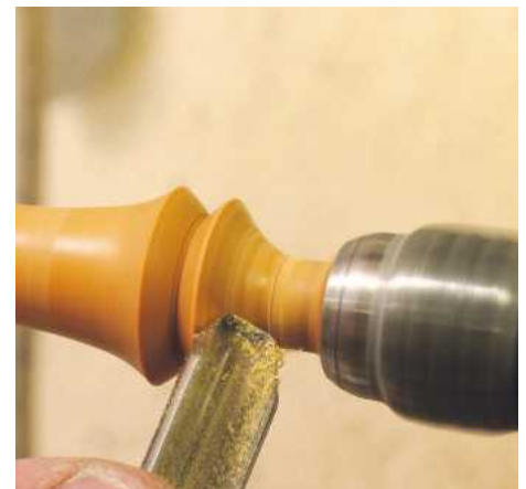
▲ Pic.27 The small gouge is used to blend a cove into the spigot. This tends to hide the hole when it's all glued together. Don't be afraid of getting right up next to the centre
